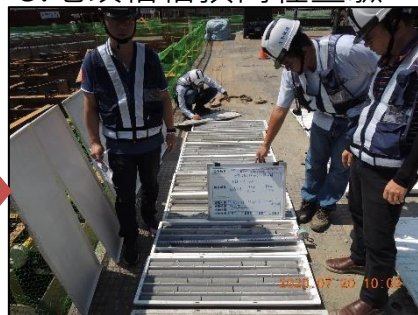
9.鑽取率、鑽心試體取樣
